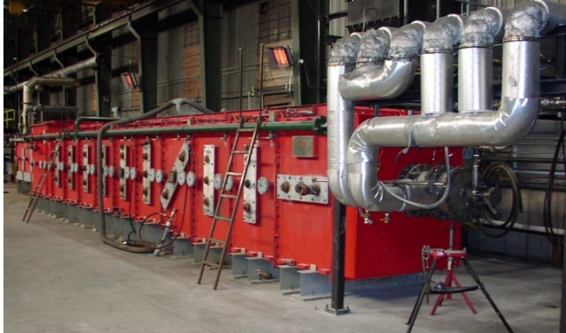
Figure 4. Photograph of the L1500 depicting the air/FGR/O 2 supply system, burner and radiant section.
