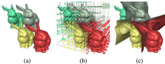
Figure 10: The method pipeline in 3D. (a) Four bunnies placed in proximity. (b) The octree with appropriately-labeled vertices. (c) The constructed GVD.
