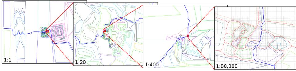
Figure 13: Path planning in 2D. We built a quadtree over hundreds of objects ranging in size and spacing over orders of magnitude. The quadtree reached level 24 before the closest spacings were resolved. The shortest-cost path between two points is shown in blue. The rightmost figure shows the quadtree in gray and GVD boundary complex in red at 80,000x magnification.
