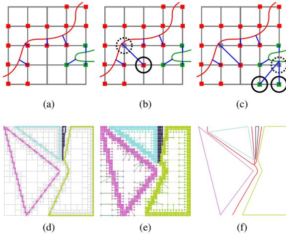
Figure 4: Wavefront expansion. (a) Portions of the surfaces of two objects. Assign every nonempty vertex an exact closest point and add the vertex to the wavefront priority queue. (b) Pop the top priority vertex (dotted circle) and push its closest point to its neighbors (circle). (c) Next iteration. (d) Initialized wavefront (as in (b)). (e) Expanded wavefront. Green lines connect quadtree vertices to computed closest points. (f) The GVD is shown in red.
