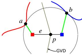
Figure 7: Computing the intersection of the GVD with quadtree edge  $e$ .  $a$  and  $b$  are closest points on objects, and  $p$  is the intersection of edge  $e$  with the GVD.
