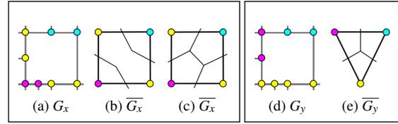
Figure 5: Ambiguous cells are detected by collapsing edges with identically labeled vertices. (a) Cell  $x$  is ambiguous because  $\overline{G}_x$  is not a simplex. (b)-(c) Two possible GVD topologies in cell  $x$  are shown. (d) Cell  $y$  is unambiguous. (e) Simplex  $\overline{G}_y$  induces a unique GVD topology.
