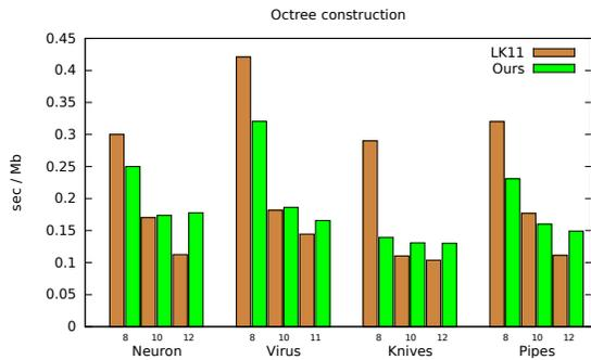
Figure 9: Comparison of our octree building to the sparse voxel octree method of Laine and Karras [LK11]. We used four datasets, each at three octree levels and compared seconds per Mb of octree memory used. Laine’s algorithm was run on a Windows 7 desktop with 3.5 GHz processor, 16 GB memory, and NVIDIA GeForce GTX 660 graphics card.
