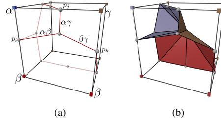
Figure 8: GVD surface generation. (a) The 2D algorithm creates GVD edges from bisectors  $\{p_i\}$  to the centroid. Each new GVD edge is given the two labels of the incident octree edge. (b) After finding the 2D GVD on its faces, the 3D cell fits triangles from 2D edges to the centroid.
