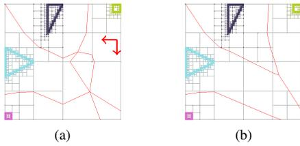
Figure 6: The effect of ambiguous cells and how they are removed. (a) The cells indicated by the arrows are ambiguous, causing the GVD to be topologically incorrect. (b) The ambiguities are resolved by recursive subdivision.
