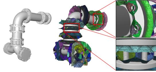
Figure 11: A pipes dataset with 392 objects and 207K object triangles. The octree was subdivided to level 10 for a total of 1.8m octree cells. The GVD separates even the nuts from the bolts (upper right).
