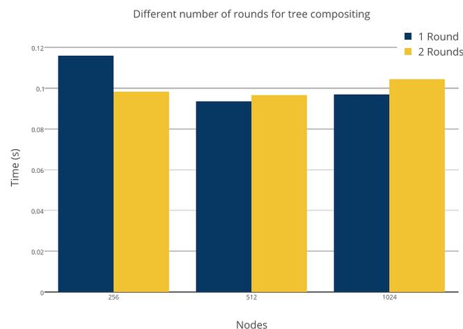
Fig. 14: Varying number of rounds for the artificial dataset for 4096x4096 on Stampede.
