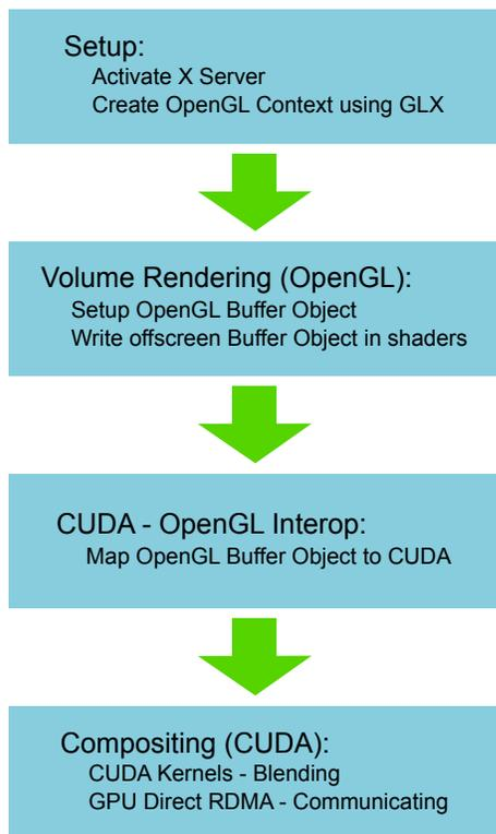
Fig. 4: Workflow for GPU rendering.
