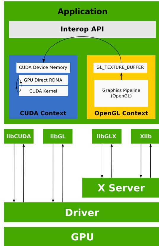
Fig. 3: OpenGL and CUDA interaction with the GPU.
