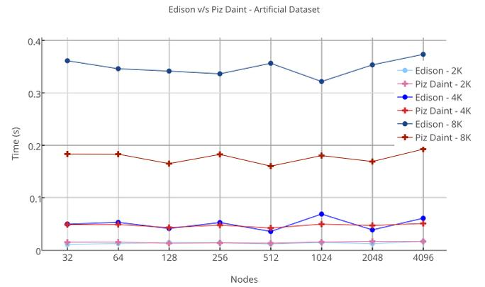
Fig. 11: Comparing scaling on Edison and Piz Daint for 4096 MPI processes.
