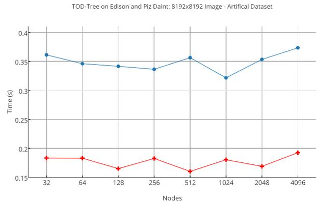
Fig. 9: Scaling for artificial dataset on Edison.
