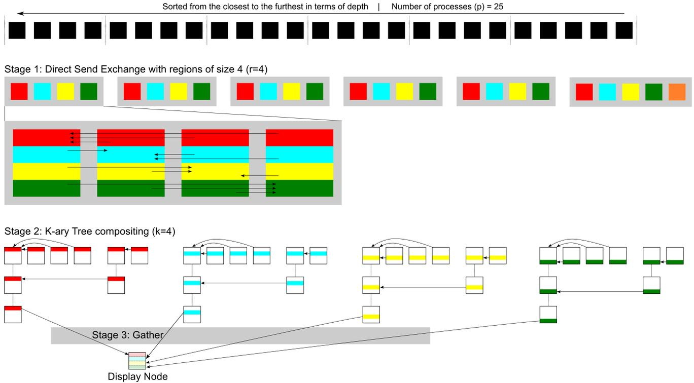
Fig. 2: The three stages of the compositing algorithm with  $r=4$ ,  $k=4$ , and the number of nodes  $p=25$ . Red, blue, yellow and green represent the first, second, third and fourth quarters of the image.
