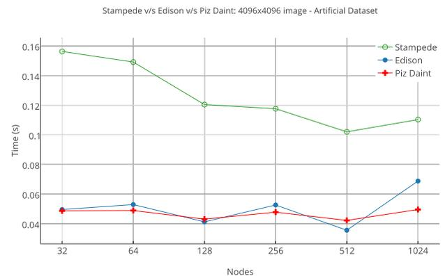
Fig. 12: Comparing Stampede and Edison for up to 1024 nodes for the artificial dataset at 4096x4096 resolution.
